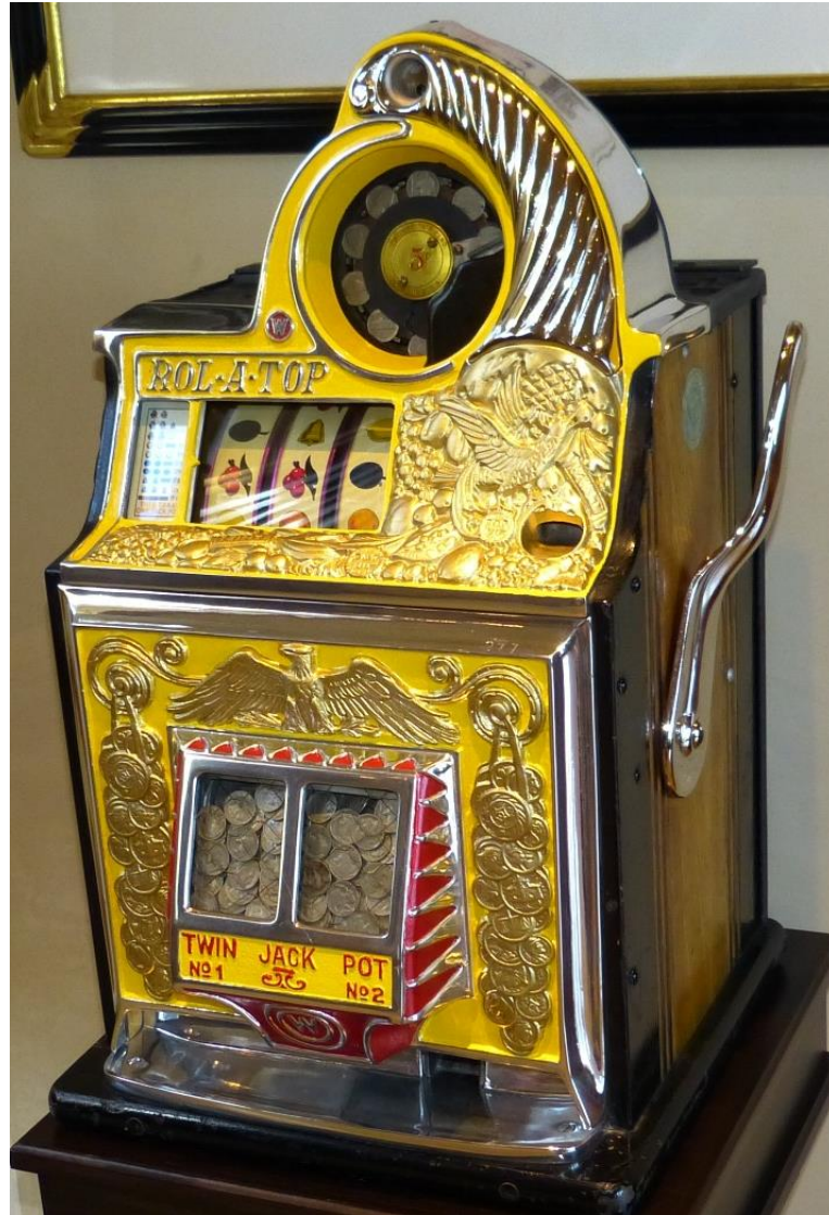
1930's Watling Rol-a-top Bird of Paradise slot machine with double jackpot, rotating coin display (fancy way of spotting slugs), but still using the iconic cherries on reel strips that go back to the original 1910 Operator Bell.
